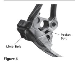
**WARNING:** DO NOTTURN THE LIMB BOLTS OUT MORE THAN THE RECOMMENDED AMOUNT. Doing so could cause the limbs to break out of their pockets and result in bodily injury.
